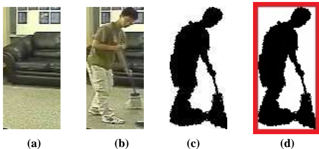
Figure 4: Foregrounding via foreground-background segmentation takes as input (a) a background image and (b) a video frame, and outputs (c) a foreground. (d) A minimum bounding rectangle (MBR) is fit around the foreground.
